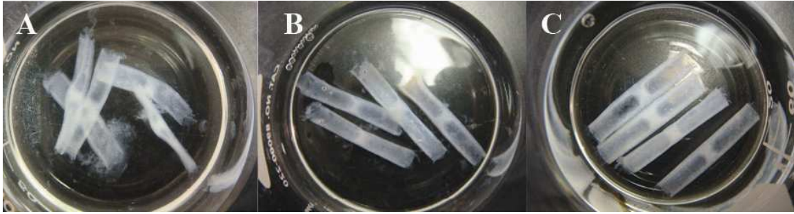
Figure 2.2 Integrity of the resulting collagen tubes made with different starting concentration. The collagen tubes made with the un-condensed collagen gel (~0.67%) were not able to maintain desired shape in vitro (A), while the tubes made with more condensed collagen gel (~1%) had observable improvement in maintaining integrity (B). A final concentration of ~1.8% collagen gel was used in the following fabrication procedure (C).
